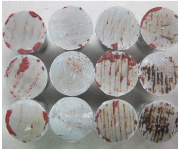
Figure 5.4: Aluminium dollies after pull of test from Resichem 530 HA 100 coating
