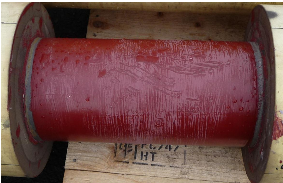
Figure 5.1 Resichem 530 HA 100 coating before exposure
