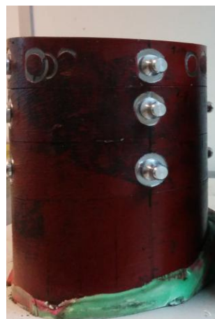
Figure 5.3: Section coated pipe with dollies attached
